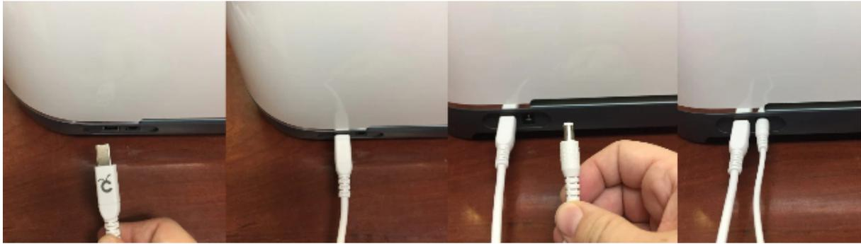
The USB cord will have a square end, plug that into the back of your machine on the left-hand side. The Cricut Logo will point downwards. The power cord has two pieces that should come preassembled. If the two pieces are not attached, simply plug one end into the other. The round end of the power cord plugs into the back of the machine on the right-hand side.
